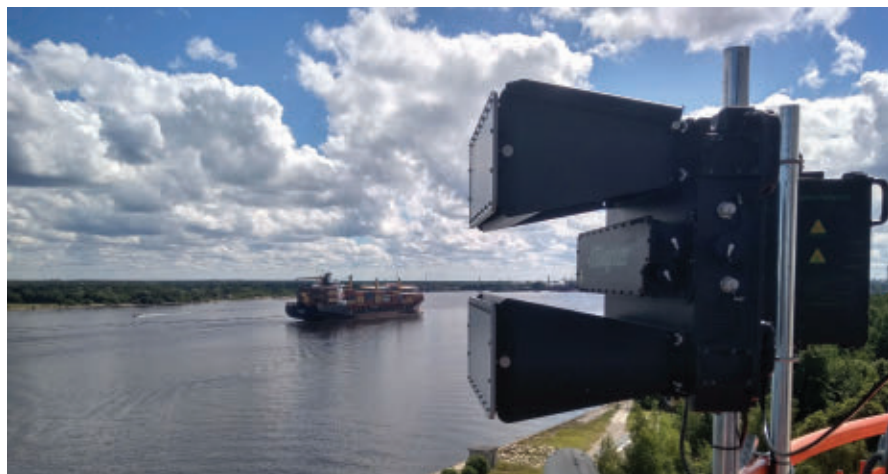
The Blighter C400 series radar can detect a small wooden boat, panga, or dory with a radar cross-section of one square meter at ranges as far as 6.8 miles, day and night, in heavy rain, dense fog, or even rough seas.
