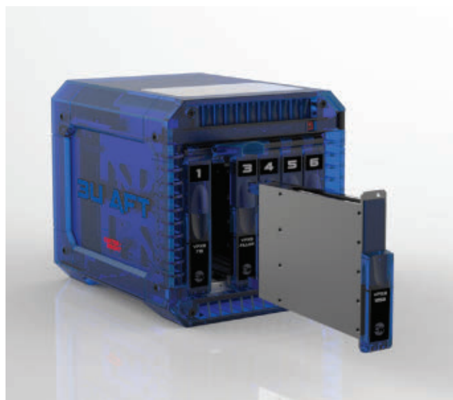
Curtiss-Wright’s Air-Flow-Through (AFT) cooling technology can dissipate more than 100 Watts per 3U OpenVPX slot.
